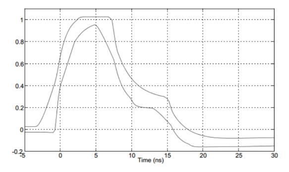
Figure 8-1 Normalized transmit templates as measured at MDI for points A, B, C, D
