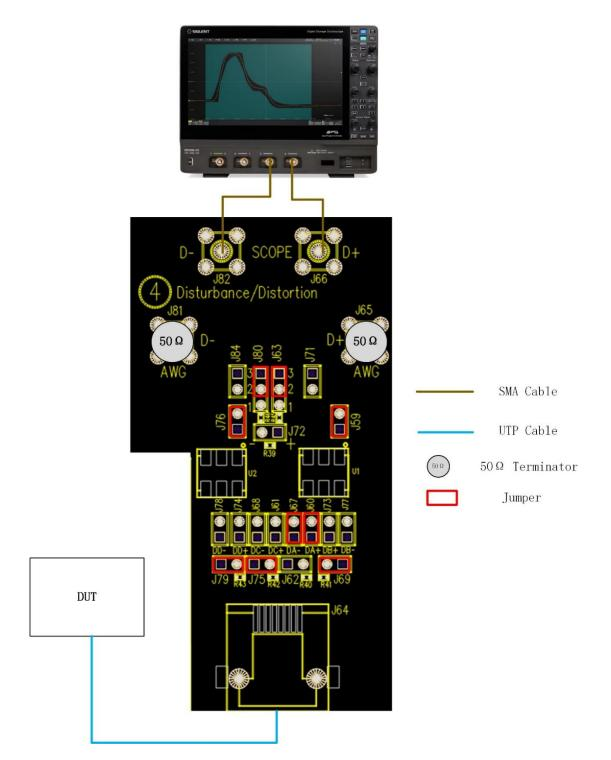
Figure 5-6 Oscilloscope measures DUT's signal amplitude which pass through the power combiners
