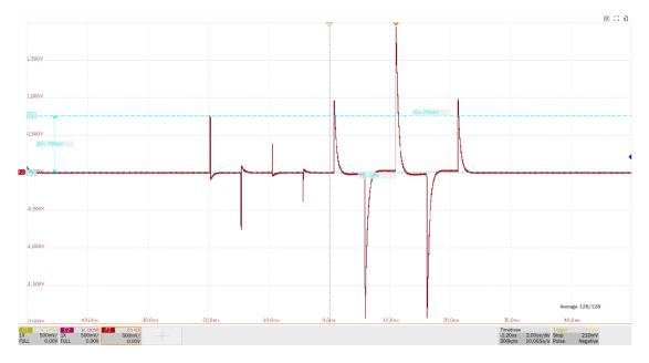
Figure 6-3 Waveform details for peak output voltage tests
