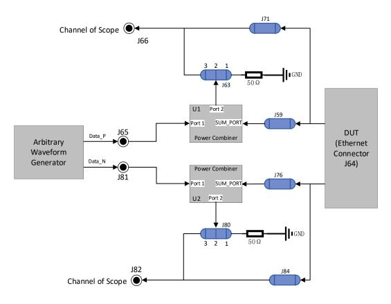
Figure 5-3 The block diagram of circuitry on section ④ of the test fixture
