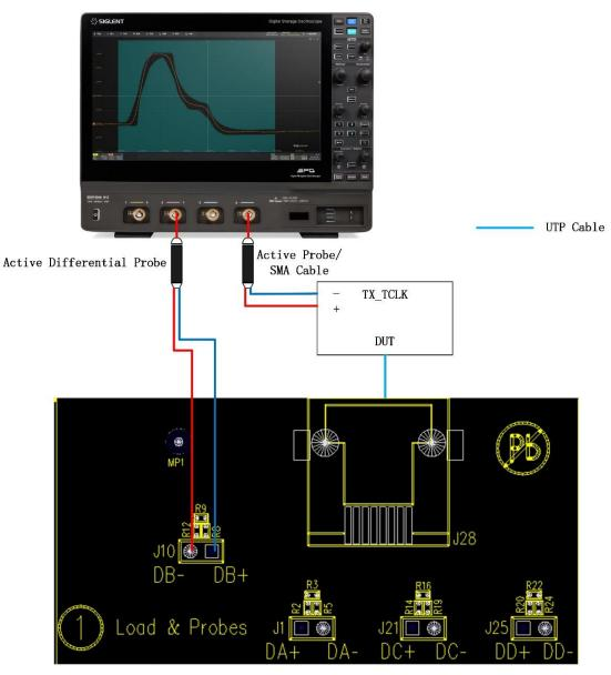
Figure 10-2 Connection of Section (1) on test fixture for Master Mode JTXOUT test
