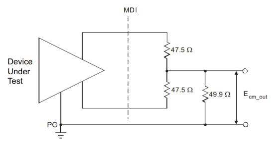
Figure 13-1 Test circuit for Common-mode output voltage
