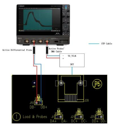
Figure 4-5 Connection diagram in the Connect menu
