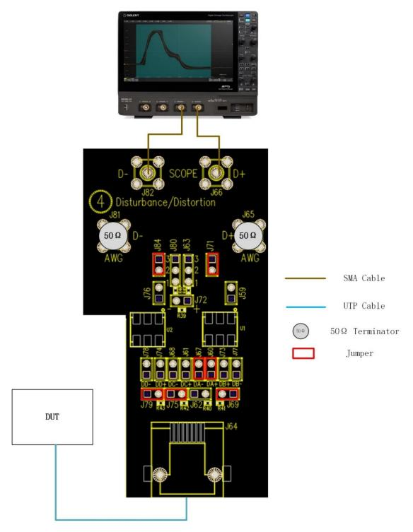
Figure 5-5 Oscilloscope measures the DUT's raw signal
