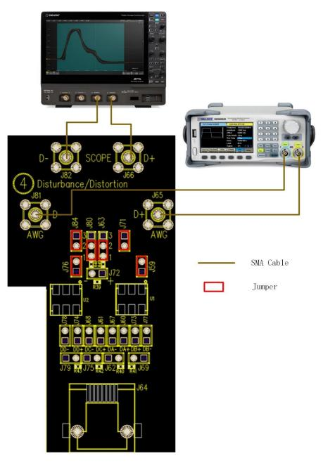
Figure 5-8 Disturber signal path calibration
