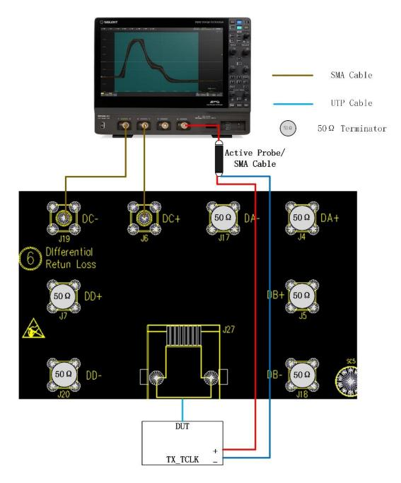
Figure 10-8 Connection of Section 6 on test fixture for Slave Mode JTXOUT test
