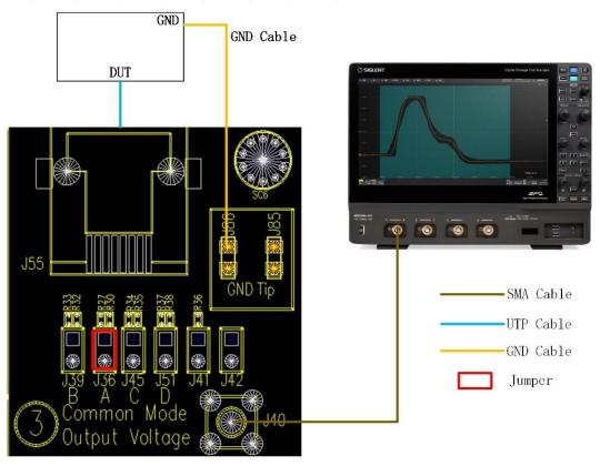
Figure 13-3 SMA cables connection in Common-mode Output Voltage
