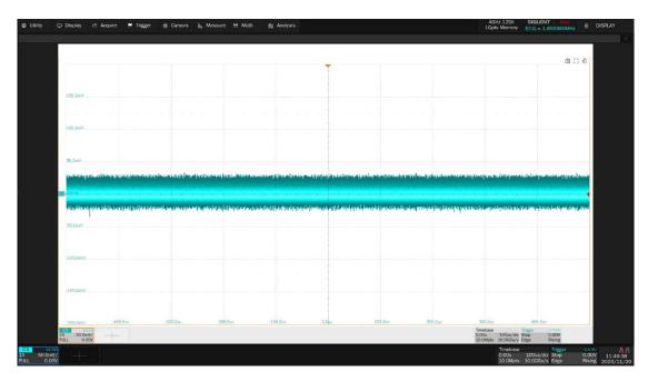
Figure 13-5 Test waveform details of common-mode output voltage
