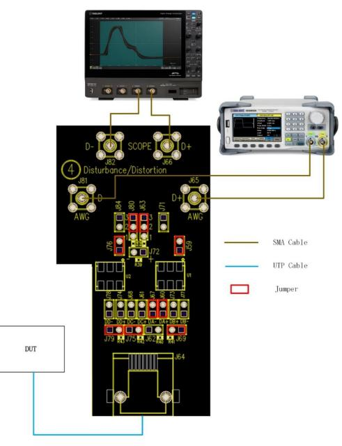
Figure 5-9 Test mode 1 and 4 test environment with disturber
