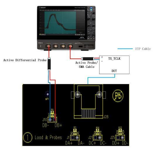
Figure 9-3 Transmitter distortion tests with TX\_TCLK and without disturber by using Section ① on the test fixture
