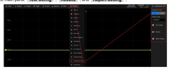
Figure 4-1 Launching 1000 BASE-T Compliance Analysis Software
