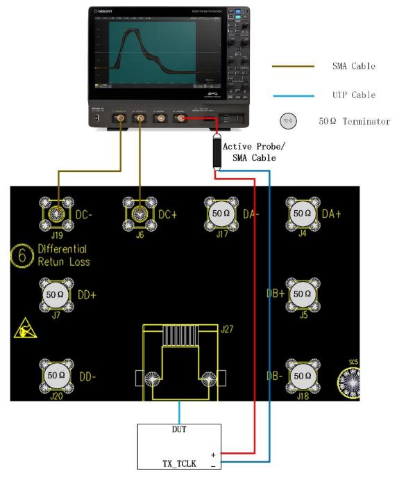
Figure 10-3 Connection of section (6) on test fixture for Master Mode JTXOUT test
