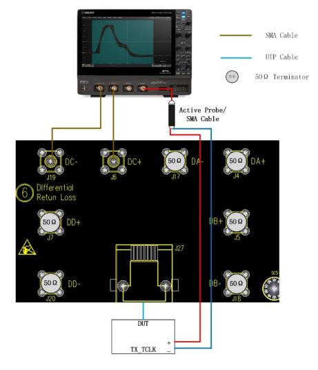
Figure 9-2 Transmitter distortion tests with TX\_TCLK and without disturber by using Section (6) on the test fixture
