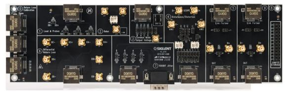
Figure 3-1 Ethernet Electrical Compliance Test Fixture Board
