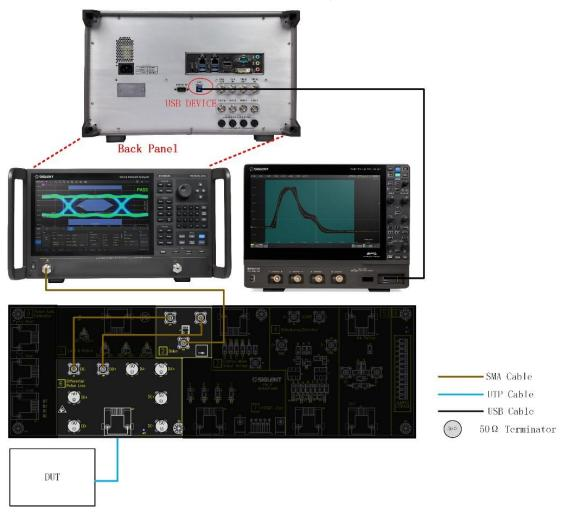
Figure 12-2 Test Environment of Return Loss
