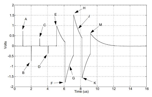
Figure 6-1 Example of transmitter test mode 1 waveform (1 cycle)
